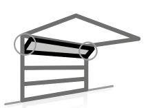
Garage ventilation feature is enabled by tilting the top panel without the need to lift the door. The bottom panel remains seated against the floor.
