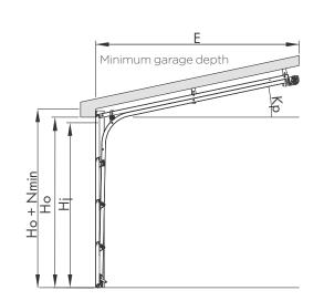
Tracks type: Inclined tracks Rear Mount Torsion
