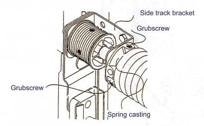
2) Thread the end of the cable into the slot of the roller bracket assembly (see item 1).
