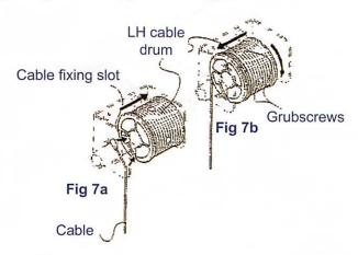
4) Undo the two grubscrews that were tightened in step 1.
